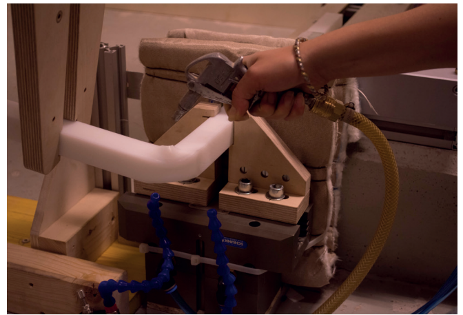
8 Air cooling after bending
